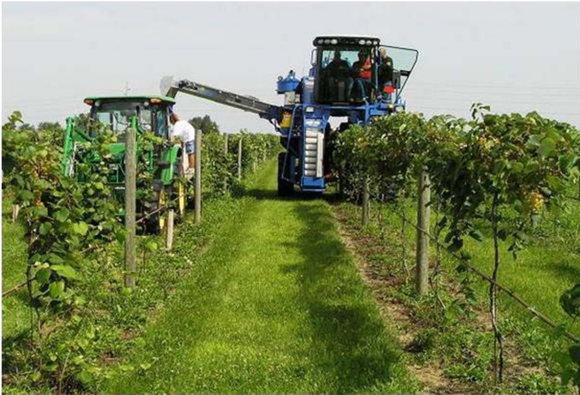
Figure 4. Korvan Self-Propelled Mechanical Wine-Grape Harvester
