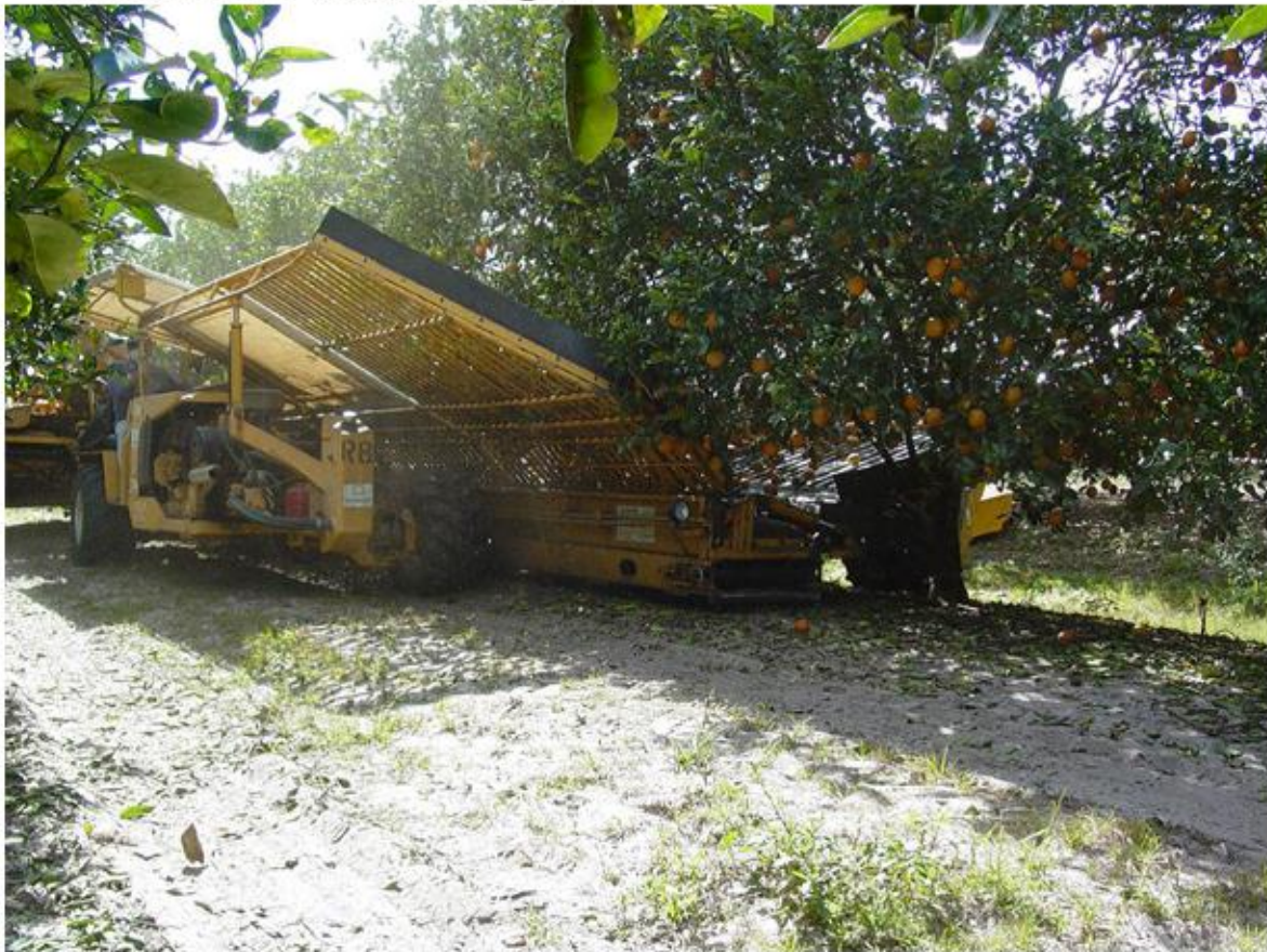
Figure 3. Coe-Collier Self-Propelled Trunk-Shaker and Catch Harvester of Florida Oranges
